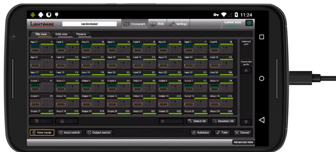
Tile View of the Crosspoint Menu of the Built-in Webpage (Displayed in a mobile device)
