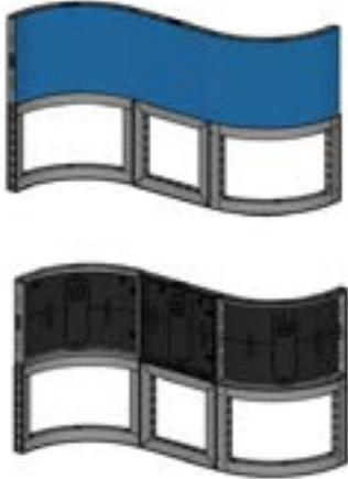
Prepare the video as described in chapter **O2 Video file**. Important to keep in mind is the amount of pixels your screens consists of. Calculate the width and height by adding the widths and heights of the cabinets in the setup.
