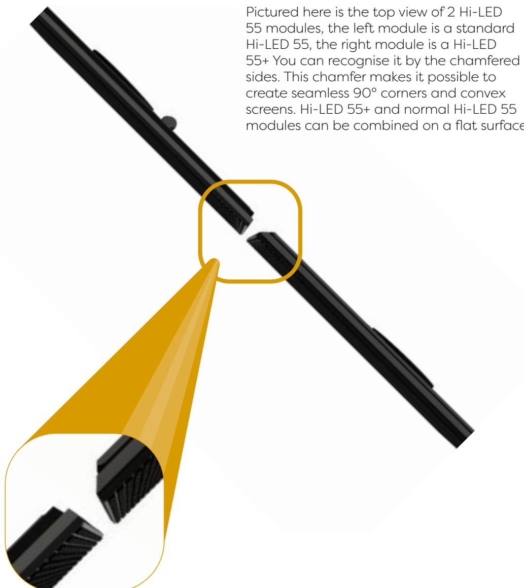
Pictured here is the top view of 2 Hi-LED 55 modules, the left module is a standard Hi-LED 55, the right module is a Hi-LED 55+ You can recognise it by the chamfered sides. This chamfer makes it possible to create seamless 90° corners and convex screens. Hi-LED 55+ and normal Hi-LED 55 modules can be combined on a flat surface
