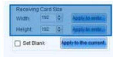
Before assigning the cabinets, set the **Receiving Card Size**. This refers to the amount of pixels in one cabinet. When using the Hi-LED 55 2.8 mm, this is 176x176 pixels. When using the Hi-LED 55 2.5 mm, this is 192x192 pixels.
