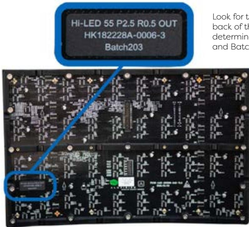
Look for this sticker on the back of the LED module to determine the pixel pitch and Batch number.
