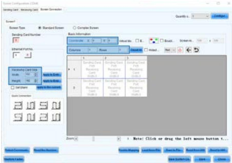
To set the correct connection, it's necessary to know the physical signal/data flow in between the cabinets. This information has to be entered in the software. In the example below the signal/data flow starts with the bottom left cabinet and runs in a vertical flow to the top right cabinet. The blue line and arrows represent the direction of the cabling.
